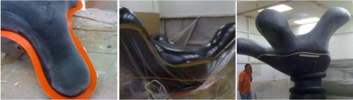
Precision OM process used to manufacture the FRP segments that make up the hand
