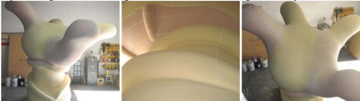
Finished Precision Board Plus plug showing bonded segments used to construct the machining block
